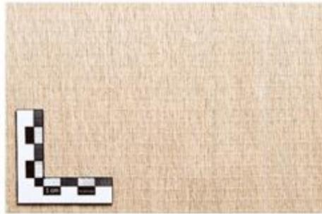
ampliTex™ 5009 non-crimp unidirectional flax fabric with fibres oriented at 0°, suitable for manufacturing of high performance composite products with low environmental impact.
