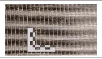
ampliTex™ 5027 fusion UD tape is a flax-carbon hybrid non-crimp tape, made of low-twist yarns. ampliTex™ 5027 is used as local reinforcement for areas subjected to severe loads or to cover for larger surfaces.
