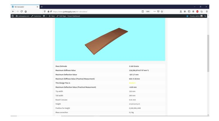
Max stiffness is 635N/mm for the glass fabric simulation. This is considered medium.
